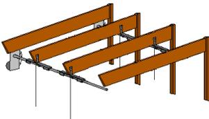
Installing two independent hoists on a wood structure allowing to straight line lift boats exceeding 8500 lbs.
