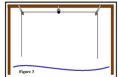
Recommended Joist Spacing: 10' to 12' apart.
