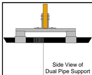
Use one section of cable for the front and one for the back. Drill a hole in the pipe and run the cable through. Cables need to run perpendicular to pipe, not at an angle. See Figure 2.
