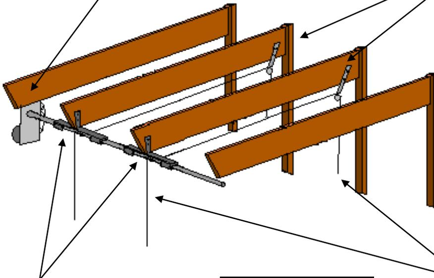
In this application the dual pipe supports will be load bearing. Each pipe support must be well greased to help eliminate unnecessary friction.
