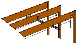
A common construction method where the boat house has two joist that are larger or doubled to carry the weight of the boat. A third joist is required to hang the hoist.
