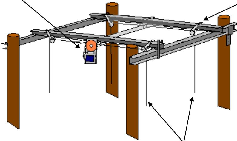
Angle the galvanized I-beam clamps (Picture 3) towards the boat at a 45 degree angle. This will eliminate unnecessary torque and help the clamps from sliding on the I-beams while being used on extreme loads. Clamps can be used on I-beams, channels or Tubing.
