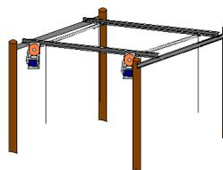
The upper structure consists of steel I-beams, tubing or channels with at least two beams running perpendicular over the slip.
