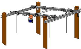
The upper structure consists of steel I-beams, tubing or channels with at least two beams running perpendicular over the slip.
