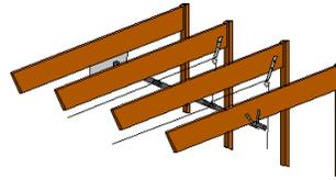
A common construction method where the structure does not have two larger or doubled joists for the lift, but has standard 2x6 or 2x8 floor joists at 16" to 24" centers. The installer uses as many joists as needed.
