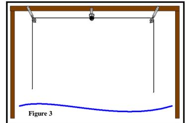
The pipe supports are designed to mount on joists that are not supporting the blocks and strap hangers. You must mount one pipe support before and after the lifting point. We also recommend using additional pipe supports every ten feet. See Figure 1.
