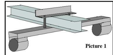
The dual pipe support for steel mounting (Picture 1) is specifically designed to line up with the BHUSA hoist hanger (Picture 2) and will not work unless used with the steel hoist hanger.
